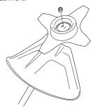
When fitting, tighten the nut in the opposite direction to the direction of rotation of the cutting attachment. To remove it, undo the nut in the same direction as the cutting attachment rotates. (CAUTION! The nut has a left-hand thread.)
